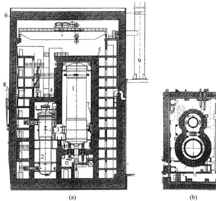
Figure 3.7 Primary system of the HTR-Module ( $200\text{MW}_{\text{th}}$ , process steam generation)<sup>[8]</sup>
