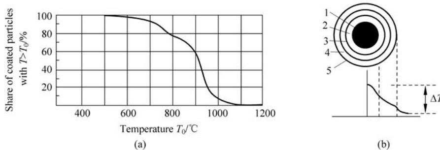
Figure 3.12 Some results of thermo-dynamic analysis of VHTR-fuel elements in normal operation
