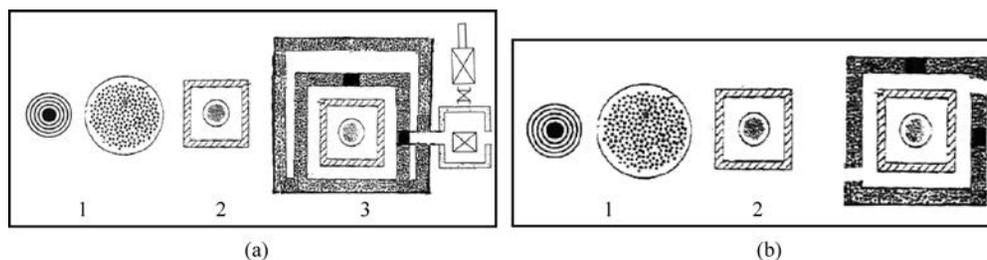
Figure 3.6 Concepts of barriers to retain fission products in the plant
