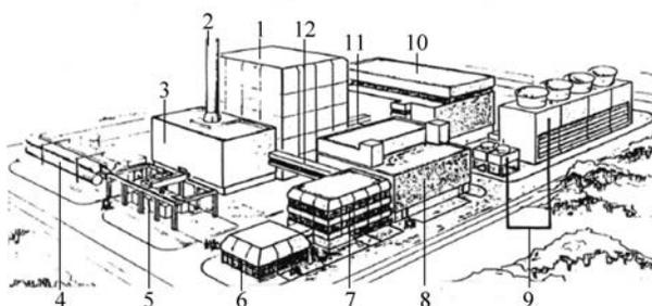
Figure 3.5 Site plan of modular reactor system with two units (example: application of steam generators without IHX)<sup>[11]</sup>
