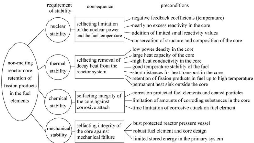
Figure 3.8 Concept of safety of modular HTR for process heat application
