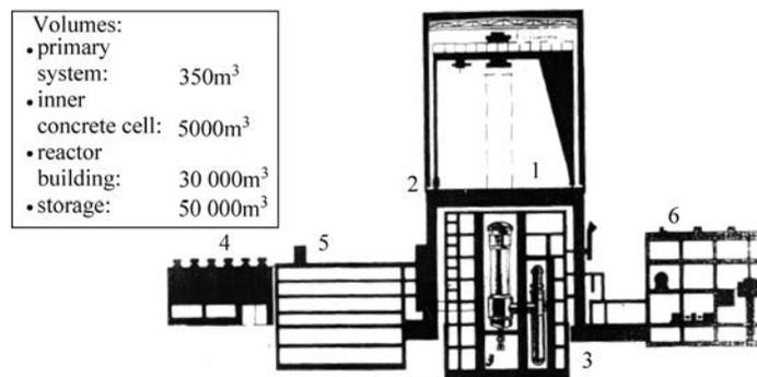
Figure 3.4 Arrangement of buildings of a HTR plant with two modular units
