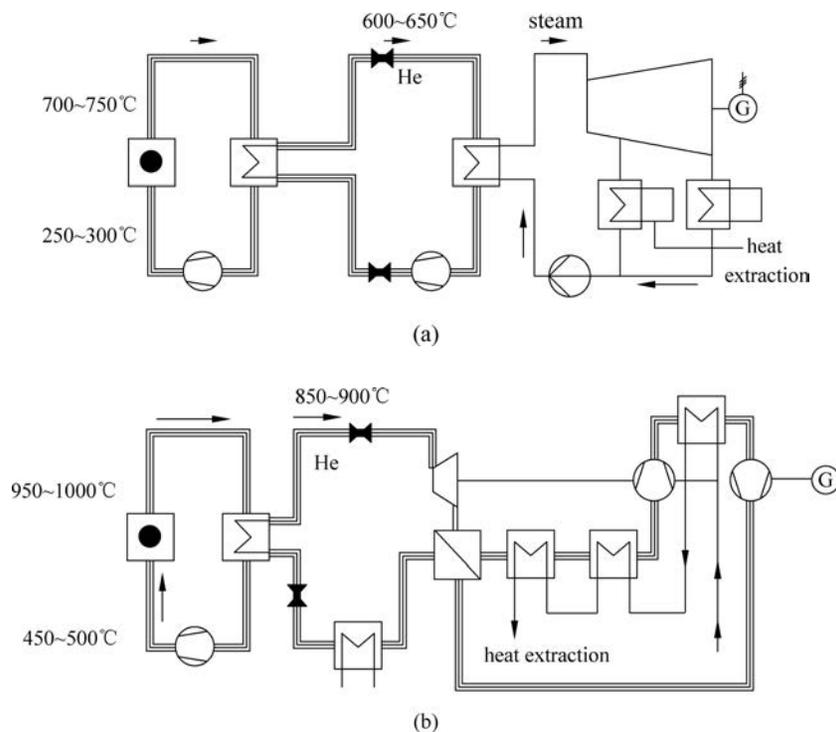
Figure 3.1 Flow sheets of VHTR-applications (with IHX)
