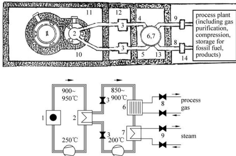
Figure 3.3 Principle arrangement of rooms for main components (example: IHX-application)
