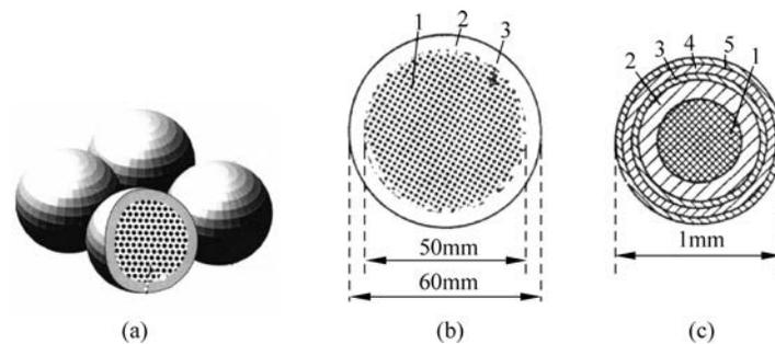
Figure 3.9 Spherical fuel elements of modular HTR (VHTR)
