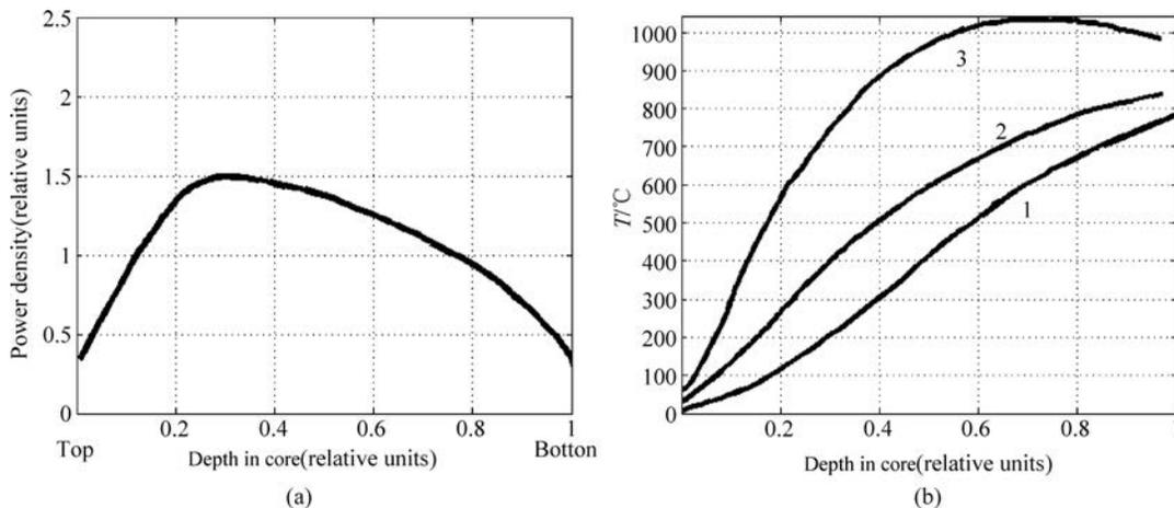
Figure 3.11 Thermo-hydraulic conditions in a core for VHTR-application ( $P_{th} = 170\text{MW}$ ;  $T_{He}(\text{outlet}) = 950^\circ\text{C}$ ; MEDUL-cycle)
