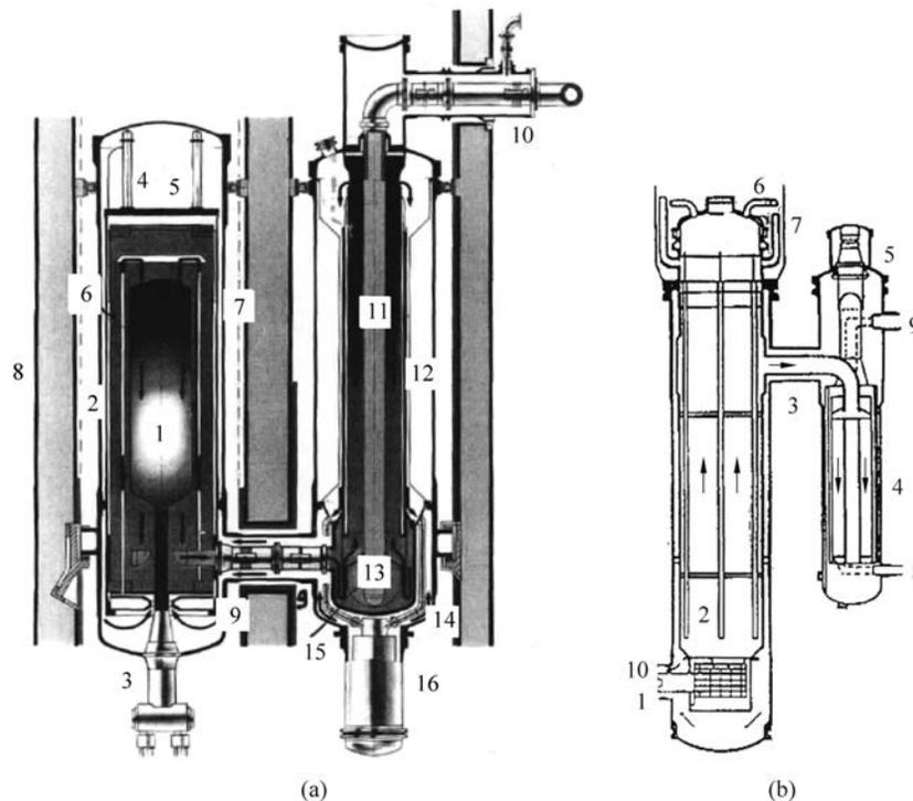
Figure 3.2 Primary system and heat utilization components for an VHTR
