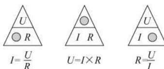
Figure 3-4 Forms of Ohm's law triangle
